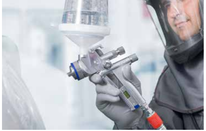
A uniform and flexibly adjustable spray fan according to the specific requirements – the SATAjet 5000 B for perfect finishes
