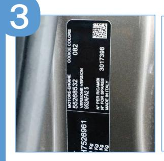
Locate and record the Colour Code of the vehicle
