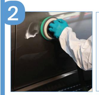
Prepare the measurement area by cleaning and then polishing
