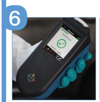
Measure 5 times by moving the Spectro, maintaining the vertical orientation
